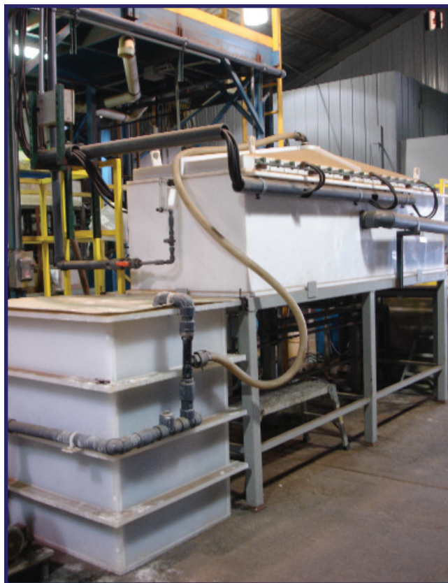
Figure 2: The rate of ROI on the EW Metals system will vary according to a particular finisher’s overall plating capacity and the specific recovery system installed. The version shown here is a 500-lb. unit.
