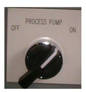
**Note:** Pump will start in soft start mode to eliminate air from the system plumbing. It will take 60 seconds to obtain full operational speed.
